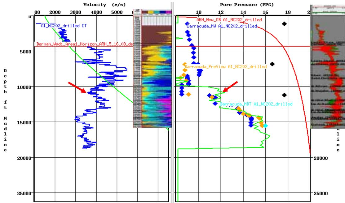
**Figure 4 Final VSP PPP update.** Calibration panel (right) showing the actual MW data (blue), the SLB PreView data (orange) and the MDT data (cyan) for the well and the predicted pressure gradient using the shale points from the VSP (green curve). The left panel is the Vp from the VSP inversion. The minima on the sonic curve are the shaley zones. Datum is mudline.
