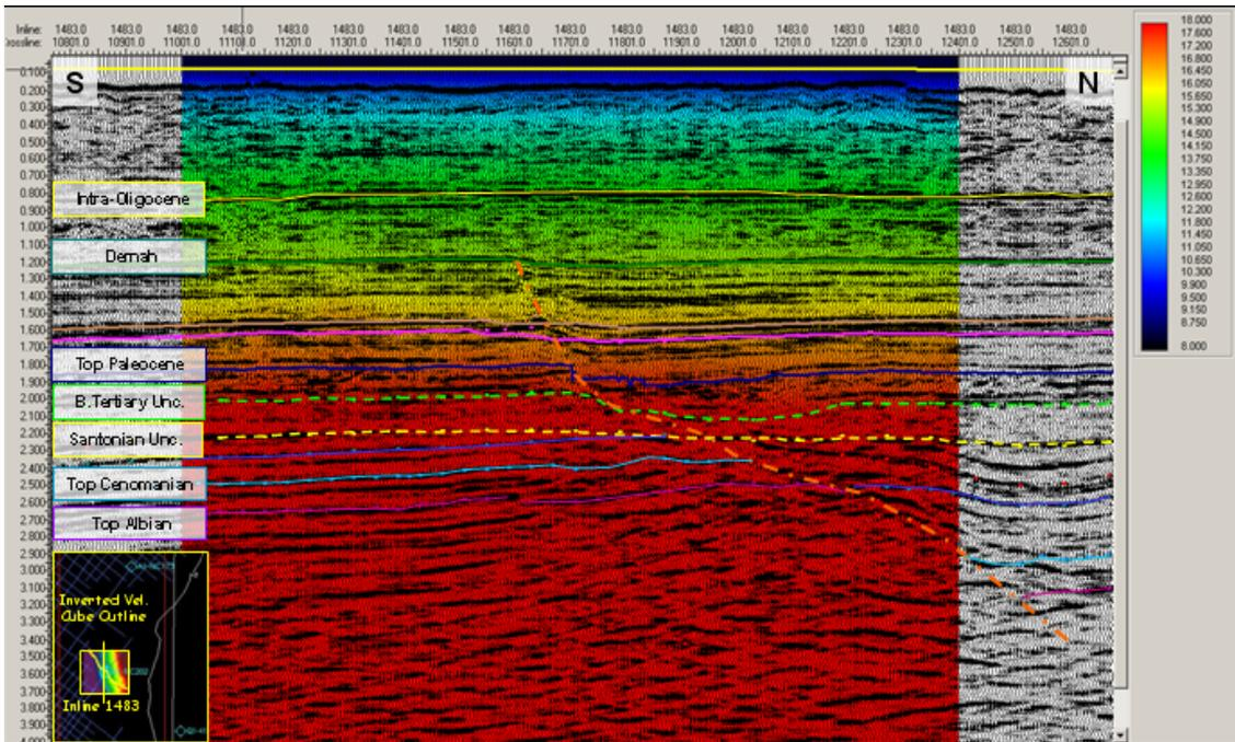
Figure 2. Fracture pressure gradient interpretation for inline 1483 using the hybrid model. The Demah horizon is shown in green. The well location is near the center of the line.
