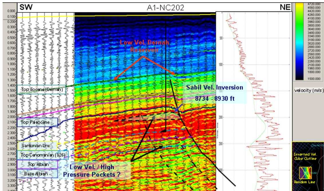
**Figure 1:** Comparison of inverted  $V_p$  using the hybrid model and smoothed shale velocity shale trend generated from the inversion at the well location results for use in pore pressure prediction.
