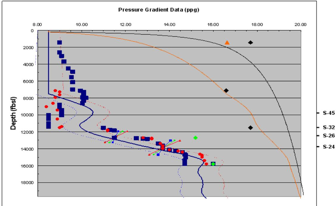
Figure 3. Original prediction from pre-drill location with actual drilling data including drilled MW (blue), PreView data (red) and MDT data (green). The MDT point at 12,772 ft is likely to be supercharged due to well killing activity and exposure to the open hole section under high MW.
