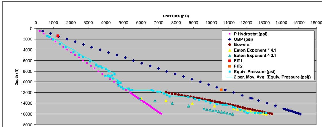
**Figure 5.** Comparison between Eaton's and Bowers Method. Instantaneous velocities derived from WL DT shale velocities ( $GR > 80$  API).
